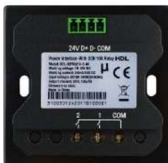
Power Interface-With 2CH 10A Relay
