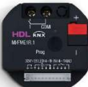
1CH 16A Flush-mounted Switching Actuator (EU)
